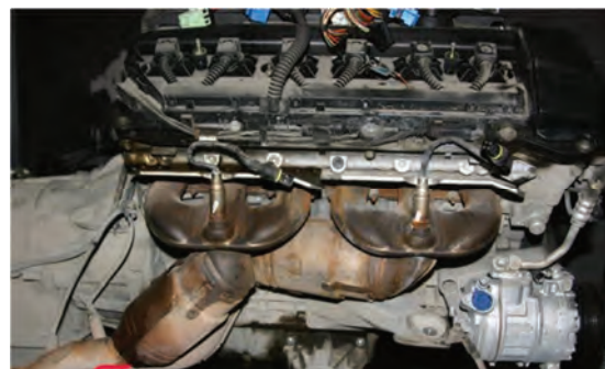
Fig. 2. Factory manifolds mounted on the engine
