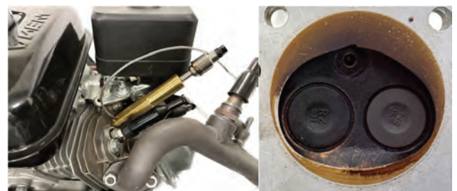
Fig. 5. Adapter mounted to the cylinder head. Note: combustion chamber view (right) does not show the additional spark plug fitting – a standard cylinder head shown
