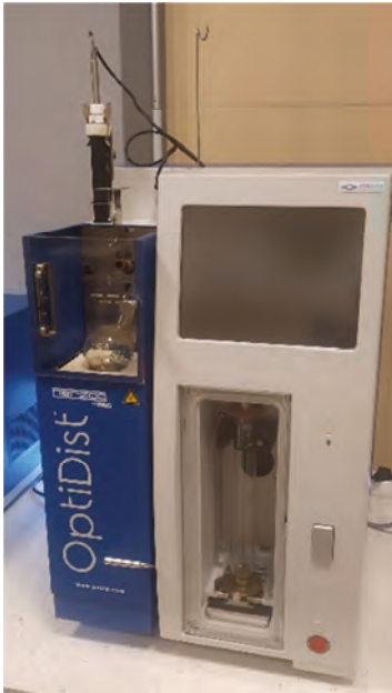
Fig. 3. Distillation analyzer OptiDist
