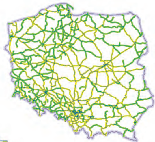
Fig. 2. Map of Polish electrified (yellow line) and non-electrified (green line) railway lines as of 18.03.2023 [8]
