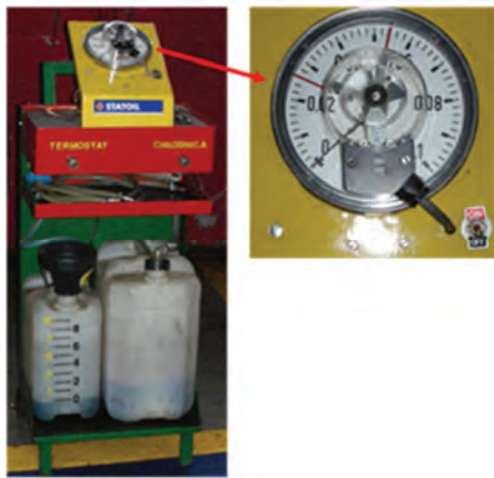
Fig. 3. The device for coolant changes and the control pressure gauge with start switch
