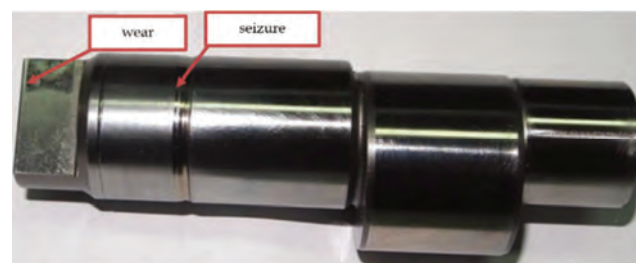
Fig. 3. Examples of damage to the pump cam shaft [10]
