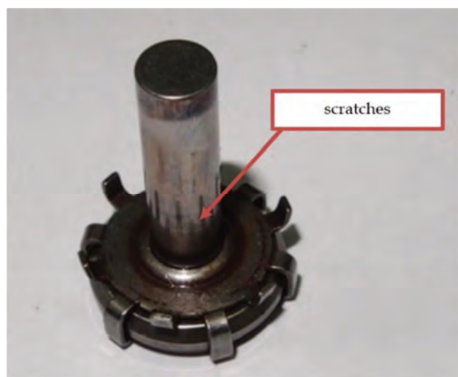
Fig. 2. Pump section piston with scratches on the side surface [10]
