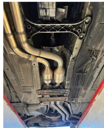
Fig. 21. The entire exhaust system after modification
