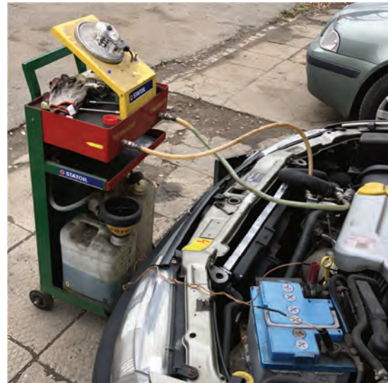
Fig. 4. The device for coolant connected to the vehicle.
