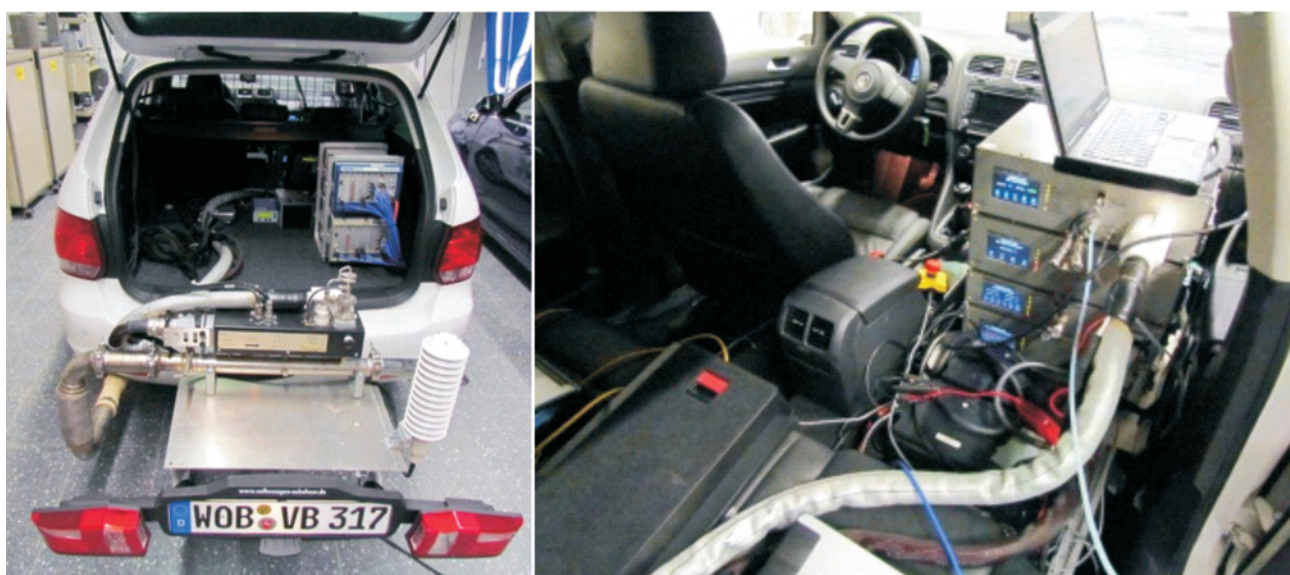
Fig. 22: Validator equipped with PEMS
