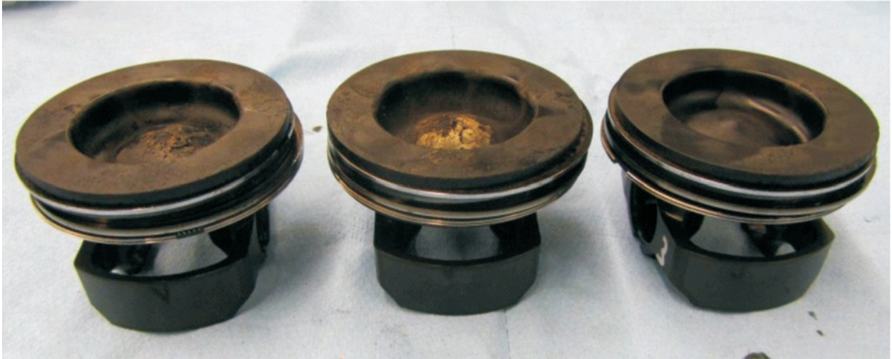
Fig. 6. Steel pistons with coking after engine testing
