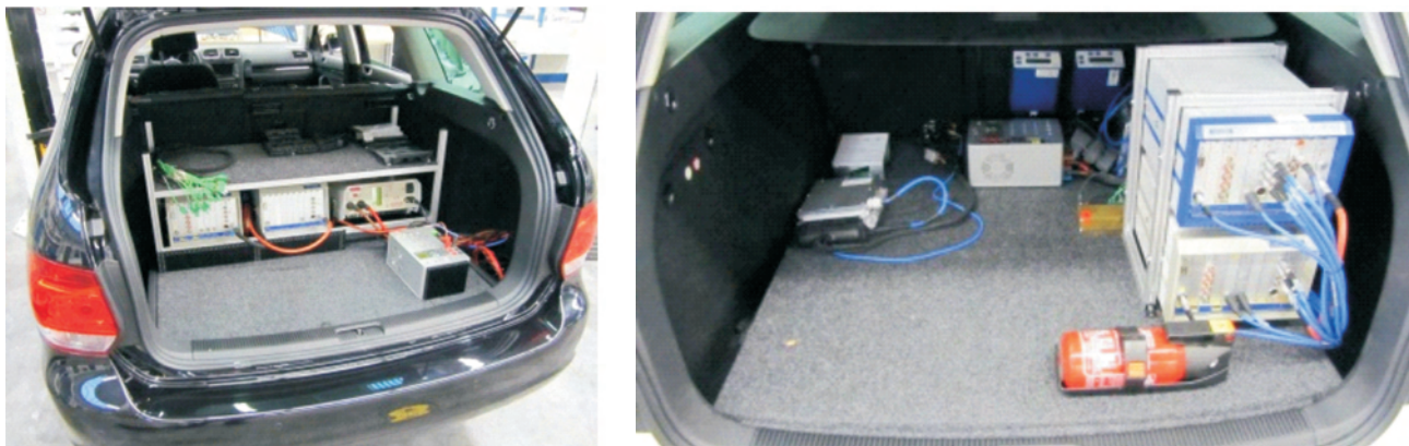
Fig. 20. Rear compartment with ES1000 and preparation for PEMS
