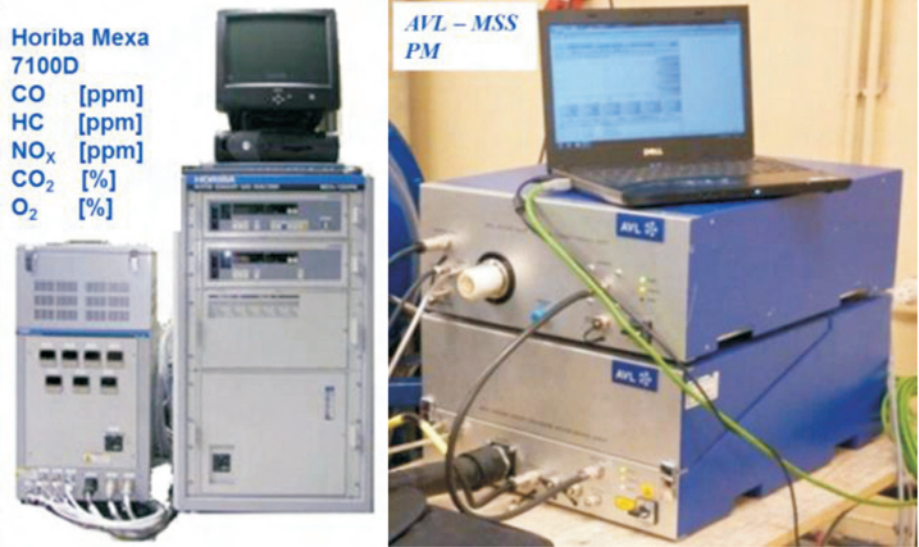
Fig. 8. Measured toxic compounds using Horiba Mexa 7100D and AVL MSS
