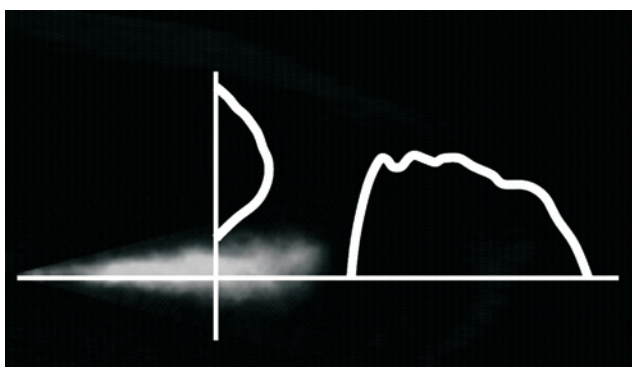
Fig. 3. Methodology of fuel distribution in cross-section and longitudinal section of fuel spray
