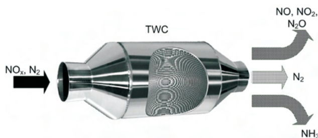
Fig. 1. A schematic of the fluxes of nitrogen and nitrogen-containing chemical species into and out of a TWC. (Note that the outputs include all the RNCs considered in this paper)
