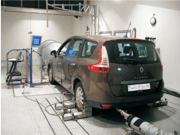
Fig. 4. Interior view of BOSMAL's exhaust emission laboratory, showing a vehicle mounted on the chassis dynamometer, together with the driver's aid (monitor) and the windspeed fan, all within the climatic chamber (-35 °C to +60 °C)
