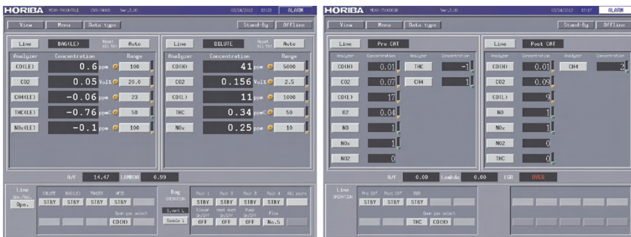
Fig. 5. Screenshots from the MEXA7000HRTLE (left) and MEXA7500DEGR (right) control systems, showing Bag LE, Diluted, PreCat and PostCat lines
