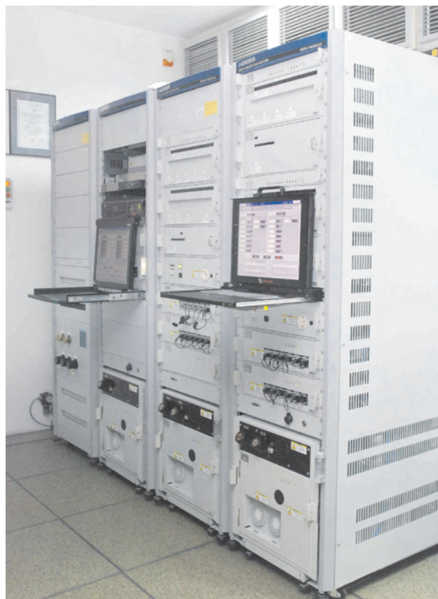
Fig. 7. MEXA-7400HRTLE (left) and MEXA-7500DEGR (right) Emissions Analysis systems
