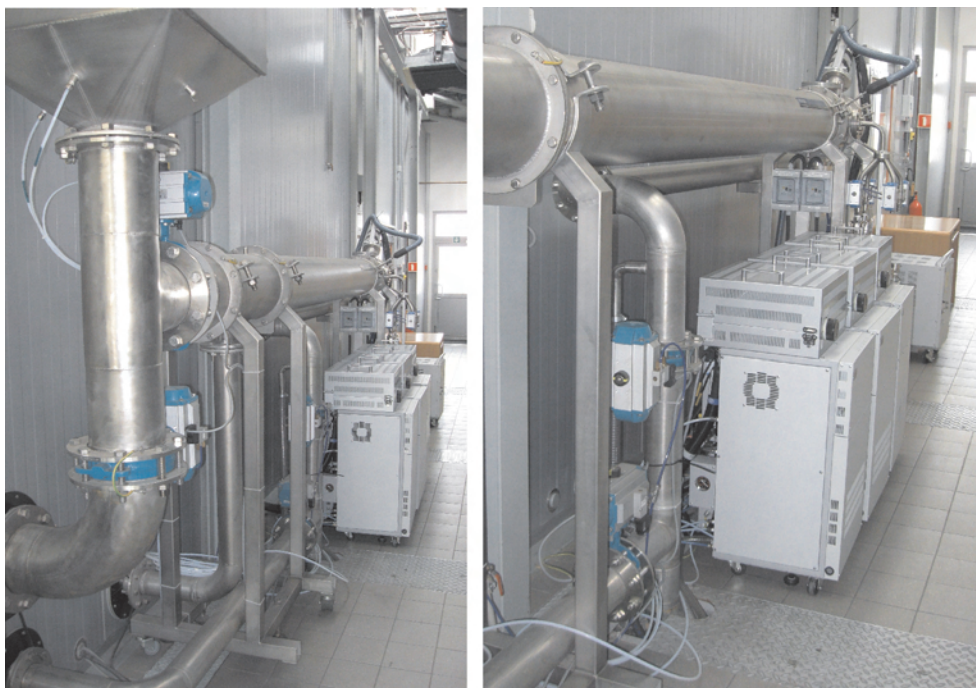
Fig. 9. Two views of the dilution tunnel (facing downstream), showing the heated OVN units for measuring emissions of THC, \text{CH}_4 and \text{NO}_x positioned under the tunnel
