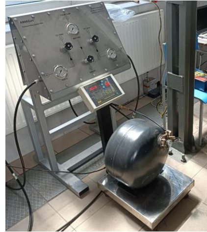
Fig. 3. Station for producing fuel blends
