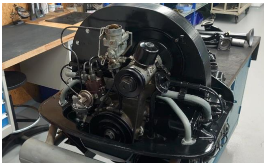
Fig. 4. The engine of a Volkswagen Type 117 car at the assembly station
