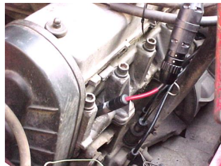
Fig. 4. MD-10B pressure sensor (a) and its connection to the spark plug hole on the engine (b)
