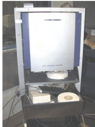
Fig. 2. The devices for the measurement of the PM content in the exhaust gas [11]: a) AVL Smoke Meter, b) AVL Micro Soot Sensor
