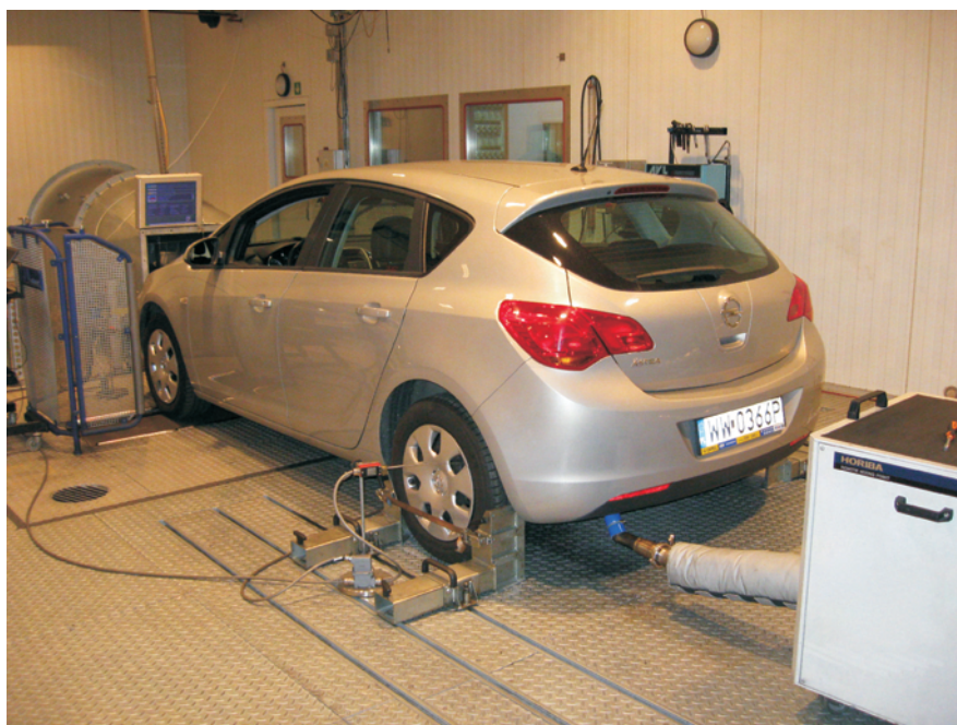
Fig. 1. Internal view of BOSMAL's climatic chamber, showing the windspeed fan and driver's aid mounted in front of a vehicle
