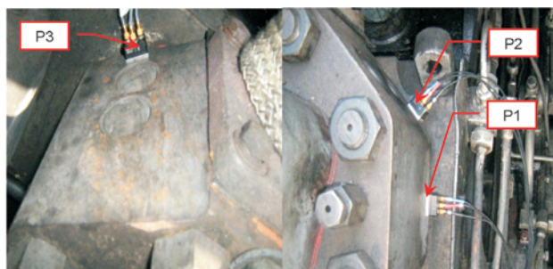
Fig. 2. Distribution of acceleration transducers on the cylinder head, engine a8C22
