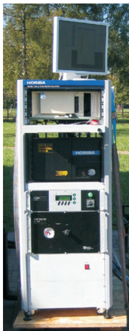
Fig. 3. Measuring system Horiba TEOM 1105
