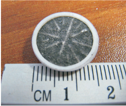
Fig. 5. Approximate dimensions of the TEOM filter; visible layer of the deposited particle matter
