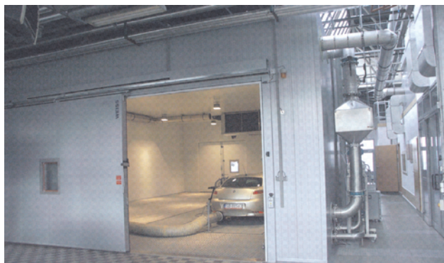
Fig. 5. BOSMAL Emission Testing Laboratory (cell 2) – external view of the climatic chamber
