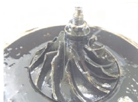
Fig. 7. Damage compressor impeller
