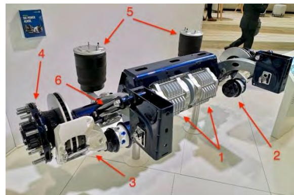
Fig. 5. Electric trailer axle with a built in electromotor for energy recuperation: 1 – electric motors; 2 – brake chamber; 3 – brake caliper and disc brake; 4 – wheel hub; 5 – air suspension bellow; 6 – shock absorber
