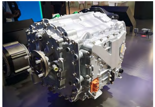
Fig. 3. Combined drive module ZF CeTrax
