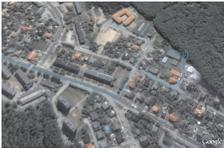
Fig. 3. The example of a route registration performed with MEREX recorder and GPS. After reaching a destination when starting, after 2–3 minute stop, some significant disturbances in GPS operation were observed
