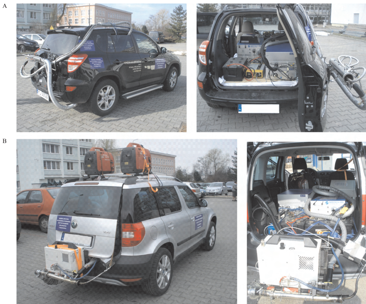
Fig. 2. Exhaust emission analyzers fitted in vehicles A and B during the tests Rys. 2. Analizatory spalin zamontowane w pojazdach A i B podczas badań
