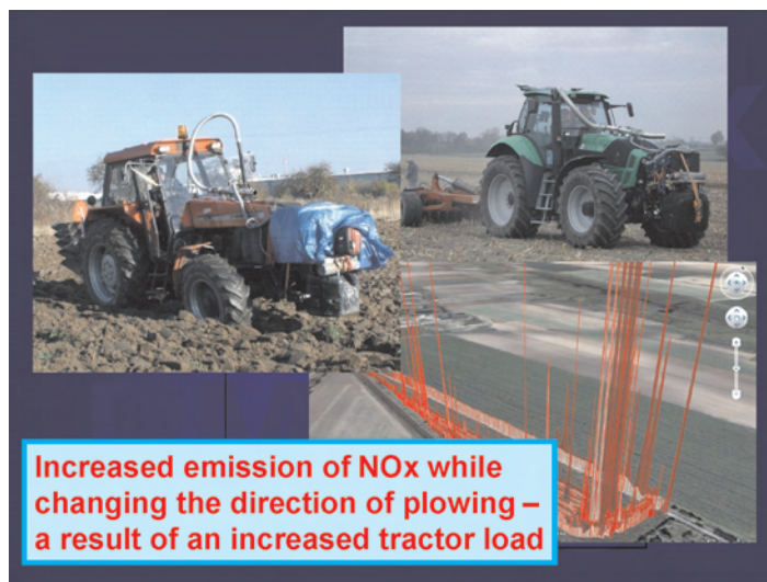
Fig. 10. Farm tractor emissions testing during fieldwork
