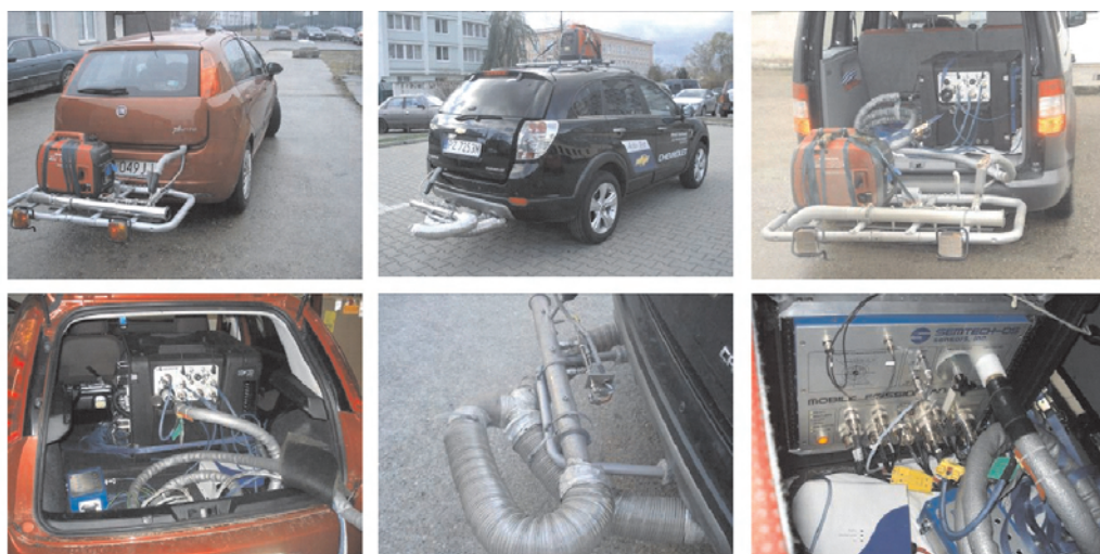
Fig. 4. Passenger vehicles during testing under real traffic conditions (fitted with various engine types: gasoline, diesel, CNG)
