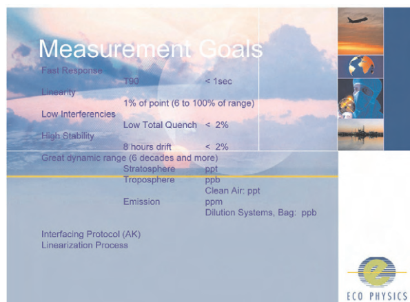
Fig. 13. Measurement goals for reliable quantification of ammonia emissions
