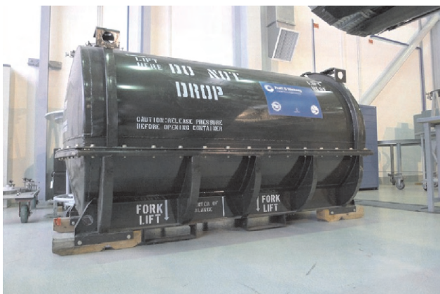
Fig. 10. Transport container for main module engine
