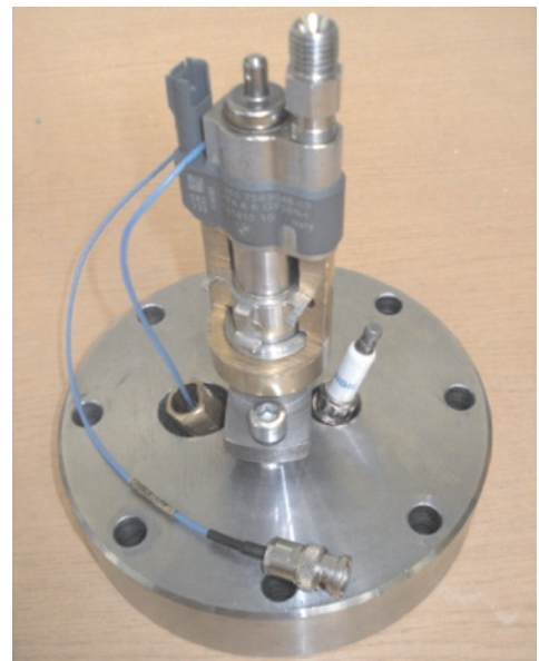
Fig. 2. Rapid Compression Machine: a) optical access to the combustion chamber, b) cylinder head with the fuel injection system and a combustion pressure sensor
