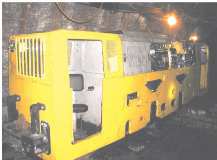
Fig. 9. Lds-100K-EMA locomotive in underground conditions [11]
