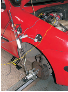
Fig. 3. The view of the wheel hub with the speed sensor and the shunt for the measurement of the starting current
