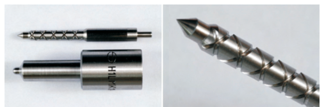
Fig. 2. Atomizer of a 359 engine with preliminary fuel treatment system and turbulizing channels
