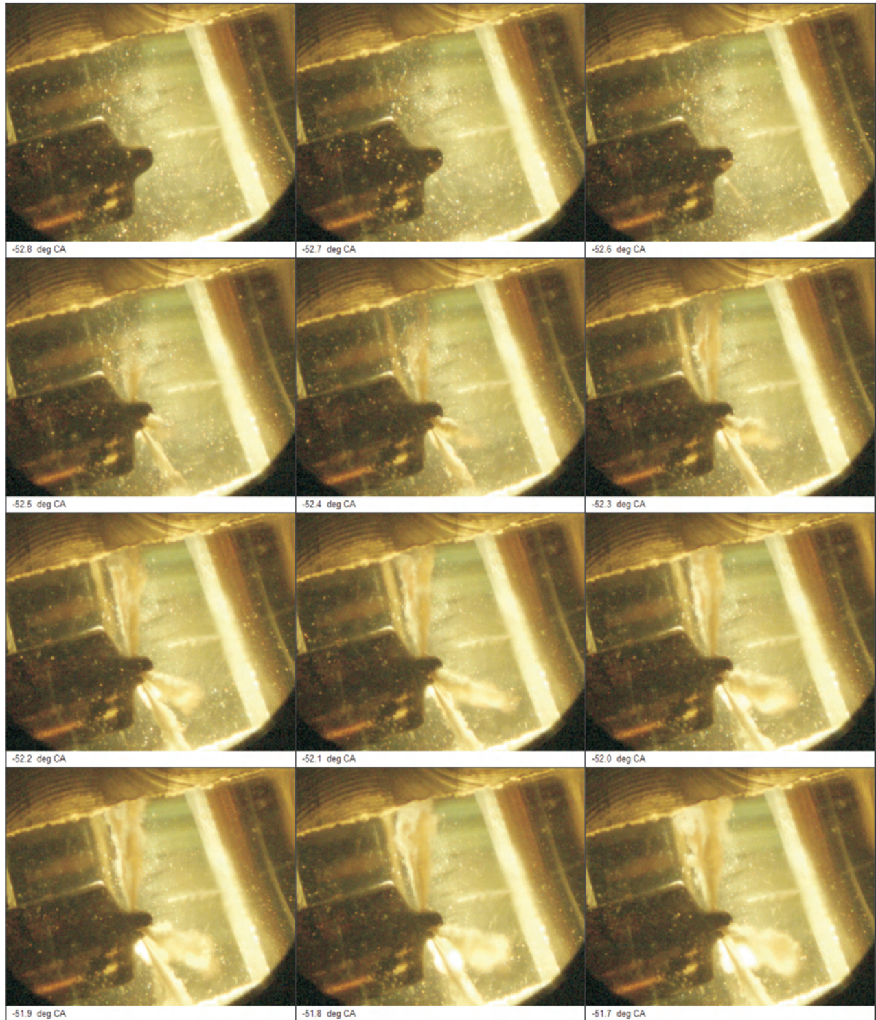
Fig. 3. Course of injected fuel stream ( p_{\text{rail}} = 100 MPa adjusted total injection duration t_{\text{inj}} = 1.0 ms, n = 600 rpm, injector Fiat) Rys. 3. Rozwój strugi wtryskiwanego paliwa ( p_{\text{rail}} = 100 MPa, czas wtrysku t_{\text{wtr}} = 1 ms, n = 600 obr/min, wtryskiwacz Fiat
