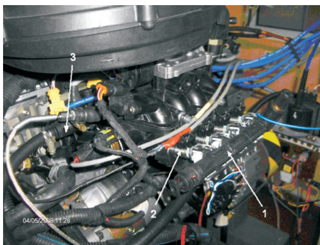
Fig. 2. Engine on a test stand: 1 – prototype fuel rail, 2 – additional injectors, 3 – original fuel rail
