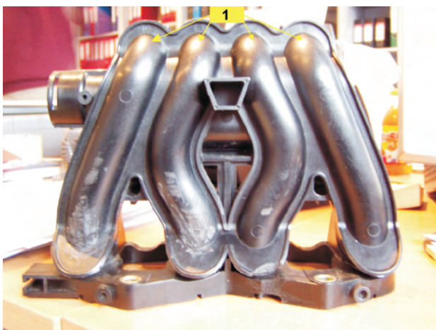
Fig. 3. Original inlet manifold by Fiat 1100: 1 – location of the additional injectors
