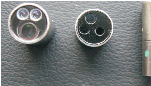
Fig. 7. Replaceable heads fitted on the end of the fibroscope: a) direction of viewing – ahead, view angle 80 degrees, b) direction of viewing – ahead, view angle 60 degrees, c) direction of viewing – sideways, view angle 80 degrees
