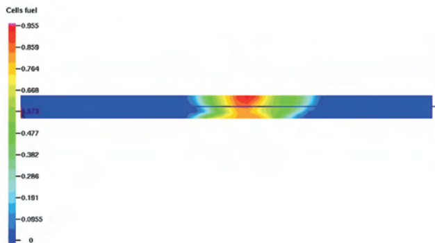
Fig. 11. Distribution of mass share of fuel vapor inside the gas conduit 13 CA after TDC
