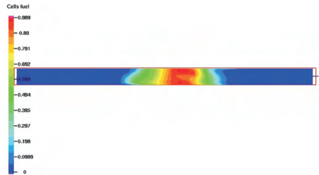
Fig. 12. Distribution of mass share of fuel vapor inside the gas conduit 49 CA after TDC
