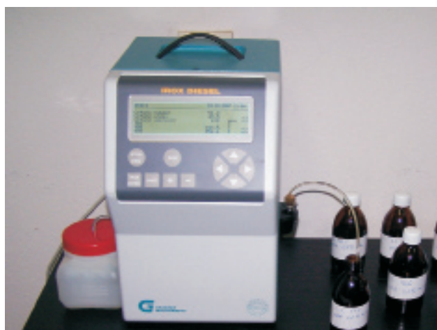
Rys. 1. Stanowisko badawcze z analizatorem paliw i biopaliw Irox Diesel Fig. 1. Experimental stand with fuel and biofuel Irox Diesel analyzer
