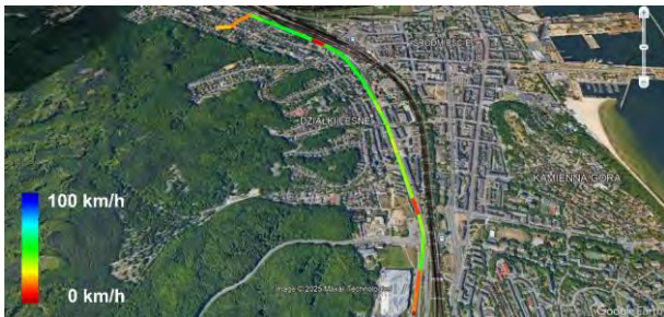
Fig. 2. Average speed distribution on route 2 over 100 m sections
