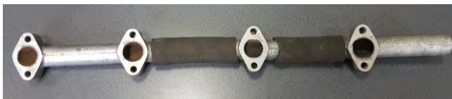
Fig. 1. Factory elements of the engine cooling system; manifold draining liquid from the cylinder block
