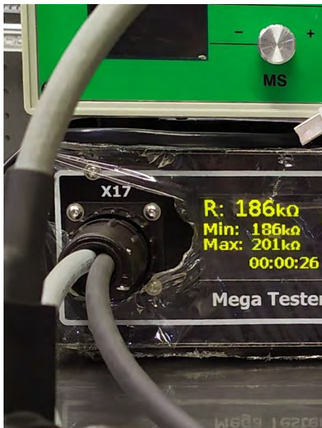
Fig. 4. Correct result of the continuous load test
