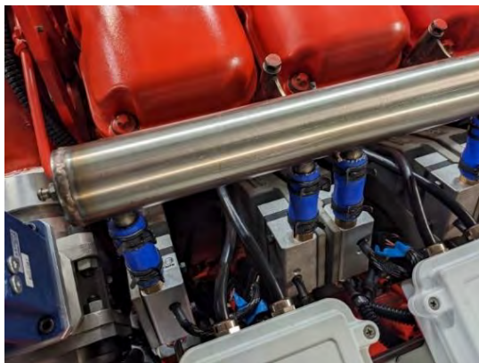
Fig. 9. A part of the fuel rail of the engine powered by gas fuels
