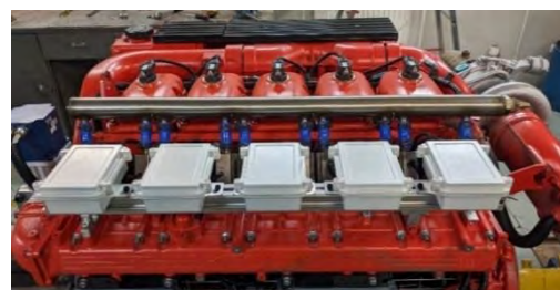
Fig. 17. Cassettes with individual injector drivers for each cylinder
