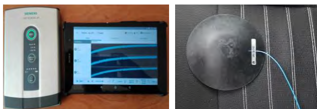
Fig. 1. Siemens LMS SCADAS XS vibration measurement system with data acquisition device – left side, three-axis seat cushion – right side
