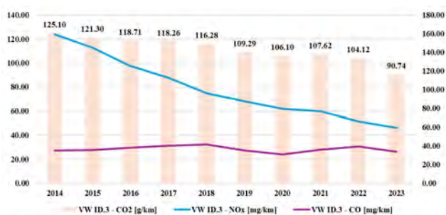
Fig. 9. Change in air pollutant emissions of VW ID.3 from 2014 to 2023, own elaboration
