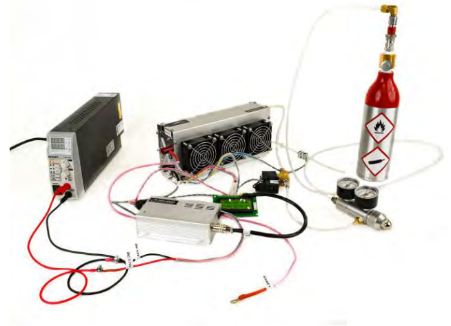
Fig. 6. Object of the research – Horizon-300W fuel cell [21]
