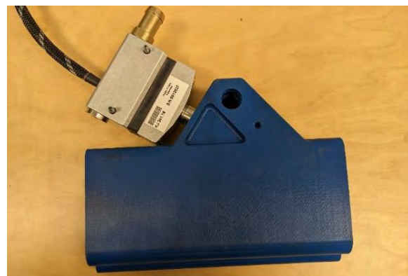
Fig. 8. Injector mounting body (in the photo – one of the prototypes printed using the 3D method from standard plastic)
