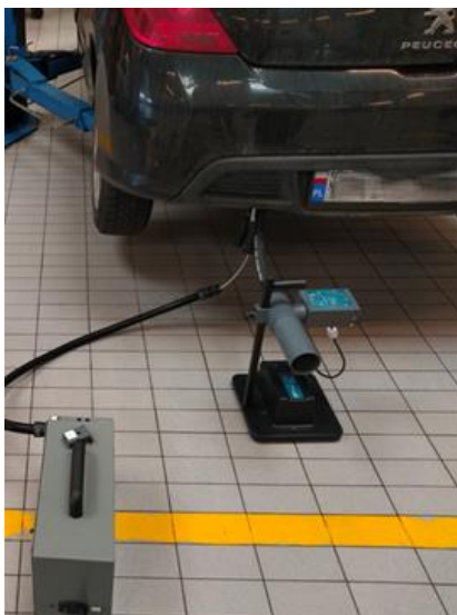
Fig. 7. Measurement of PN and PM from the exhaust pipe
