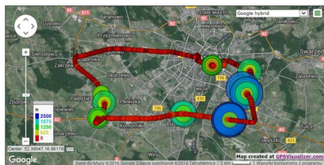
Fig. 4. NO x concentration recorded during tests for the gasoline engine vehicle (visualized along the test route)
