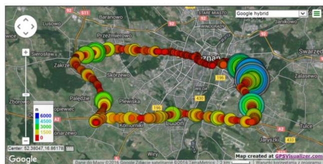
Fig. 3. CO concentration recorded during tests for the gasoline engine vehicle (visualized along the test route)
