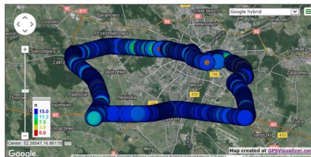
Fig. 5. CO 2 concentration recorded during tests for the gasoline engine vehicle (visualized along the test route)
