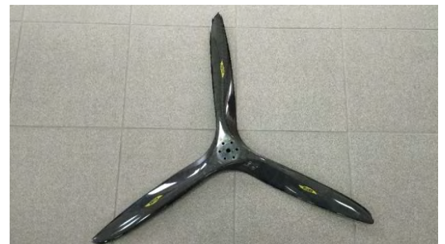
Fig. 15. Biela 32/12 3-blade propeller – view
