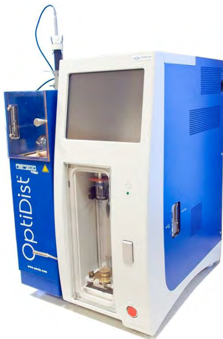
Fig. 2. OptiDist distillation apparatus used to perform atmospheric distillation tests
