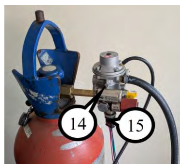
Fig. 3. Range extender equipment, continued: 14 – gas reducer; 15 – combi pressure/temperature sensor for H 2 consumption calculation
