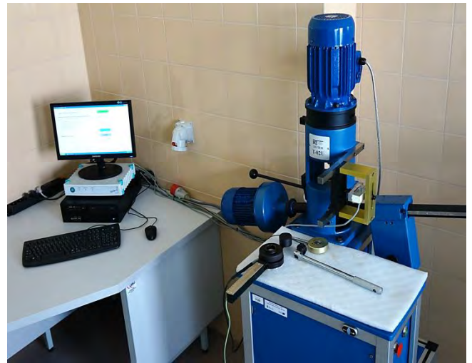
Fig. 3. View of the test stand for lubricity evaluation with the T-02U four-ball apparatus
