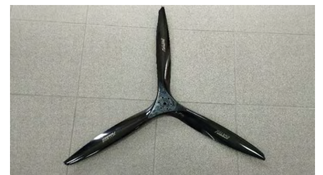
Fig. 17. Falcon 32/13 3-blade propeller – view
