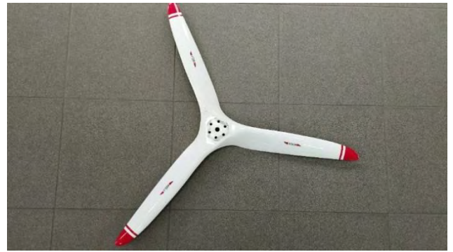
Fig. 13. Biela 32/14 3-blade propeller – view
