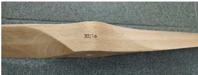
Fig. 10. Fiala 32/16 2-blade propeller – propeller geometry design
