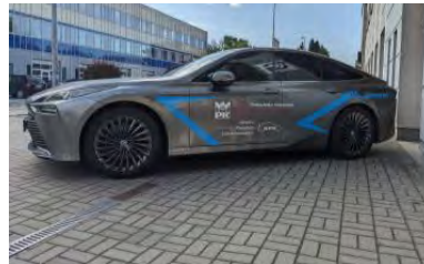
Research vehicle powered by hydrogen fuel cells (PEM)
