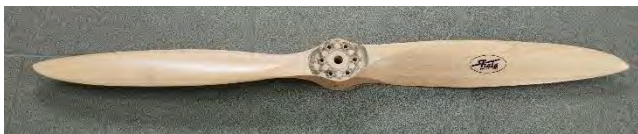
Fig. 9. Fiala 32/16 2-blade propeller – view
