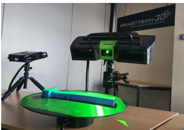
Fig. 3. Scanning of intake manifold castings with the SMARTTECH Micron3D Green Stereo scanner
