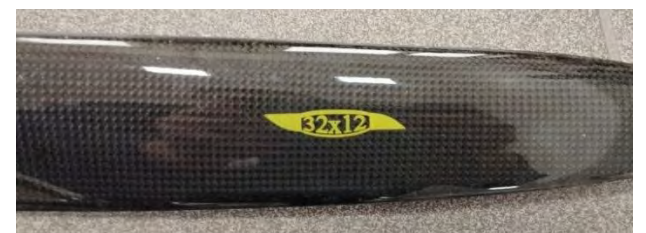
Fig. 16. Biela 32/12 3-blade propeller – propeller geometry design
