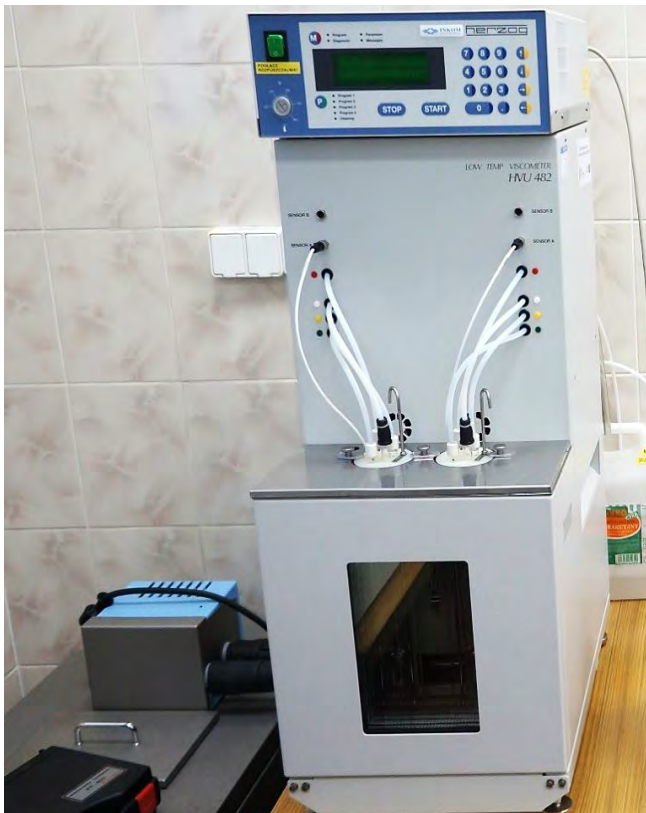
Fig. 2. HVU 482 apparatus for determining kinematic viscosity
