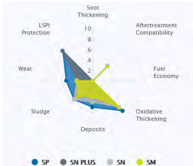
Fig. 1. API spark ignition standards [13]
