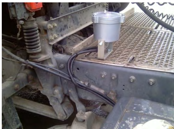
Fig. 5. a) View of the additional tank with a fuel microfiltration insert on the truck b) view of the tank with the KleenFuel insert with fuel lines [fot. Ł. Kubacki]
