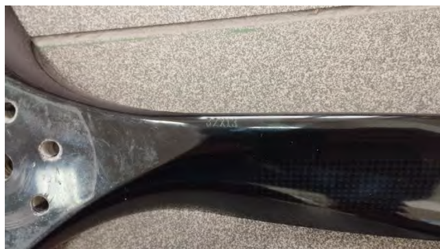
Fig. 18. Falcon 32/13 3-blade propeller – propeller geometry designation
