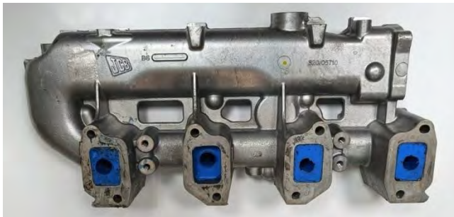
Fig. 2. Intake manifold filled with molding silicone
