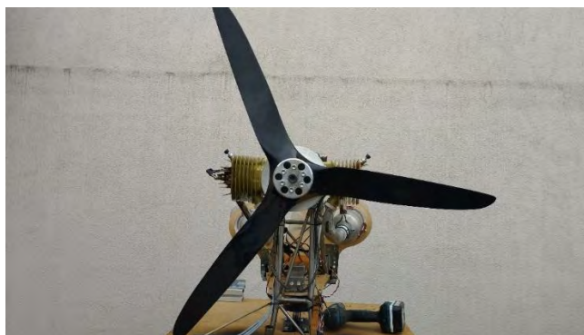
Fig. 5. 3-blade propeller made of carbon fibre
