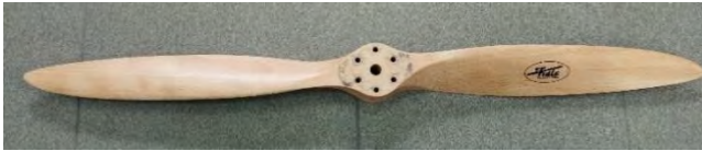
Fig. 7. Fiala 30/18 2-blade propeller – view
