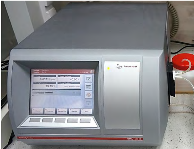
Fig. 1. DMA 4500 M apparatus for density determination
