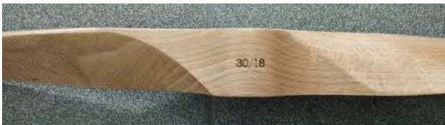
Fig. 8. Fiala 30/18 2-blade propeller – geometry design
