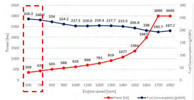
Fig. 4. Power and specific fuel consumption of the CAT C175 3000 kW engine as a function of speed
