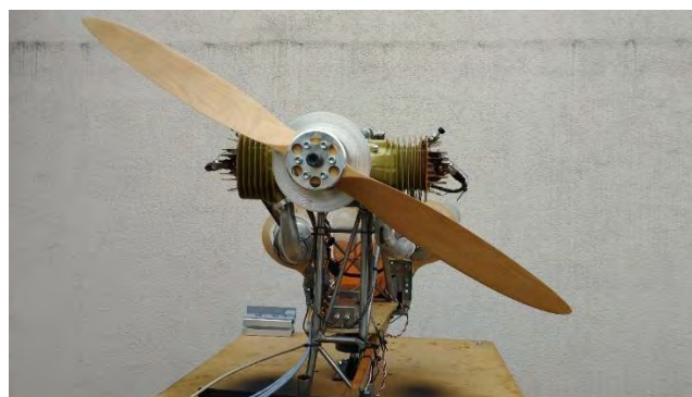
Fig. 6. 2-blade propeller made of wood
