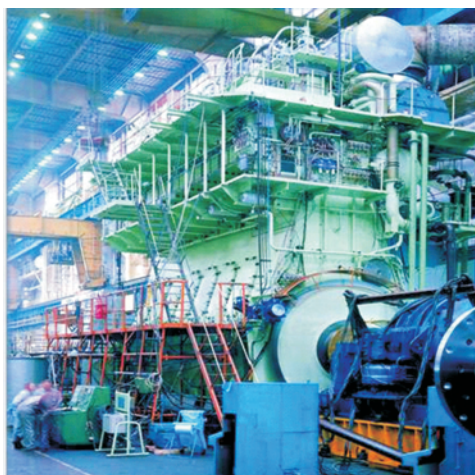
Fig. 5. MAN B&W 7S70MC-C engine during a sign-off test
