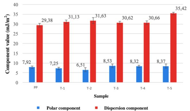
Fig. 1. Free surface energy components values for samples
