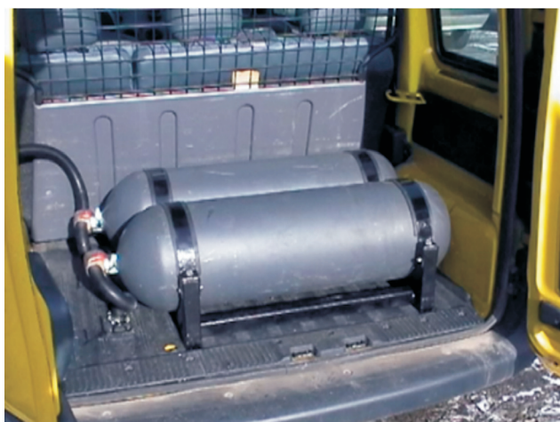
Fig. 4. Steel CNG tanks, p_{\max} = 20 \text{ MPa}
