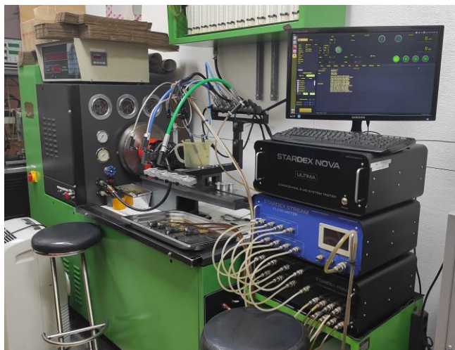
Fig. 2. 12PSB test bench with a Stardex test kit
