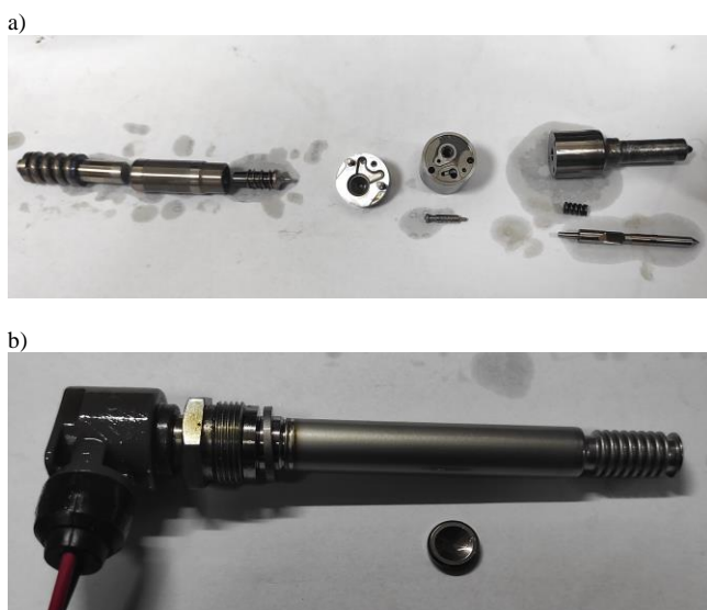
Fig. 5. Examples of assemblies after disassembly: a) hydraulic booster, valve, nozzle, b) piezoelectric actuator
