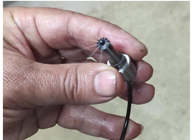
Fig. 6. Checking the patency of the nozzle openings
