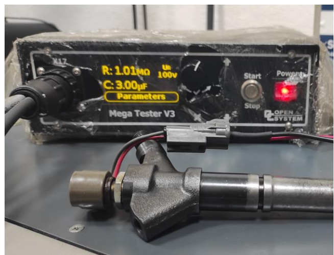
Fig. 4. Testing of the electrical parameters of the fuel injector
