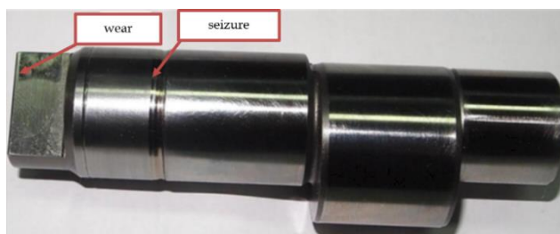
Fig. 3. Examples of damage to the pump cam shaft [10]
