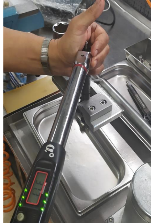
Fig. 7. Tightening the nut with a torque wrench
