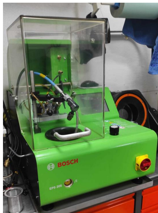
Fig. 1. View of the Bosch EPS 205 test bench
