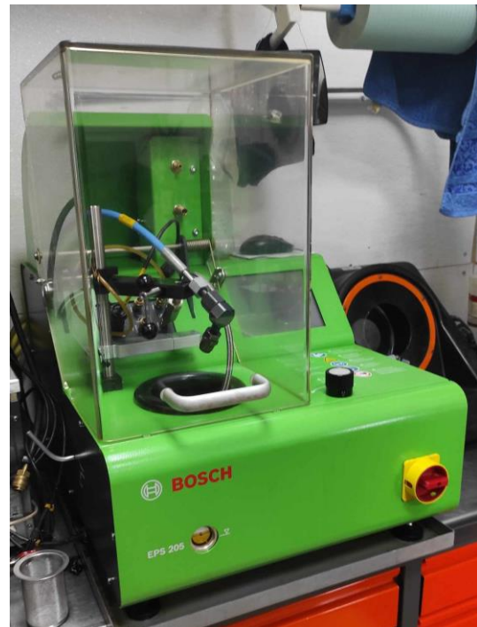
Fig. 1. View of the Bosch EPS 205 test bench
