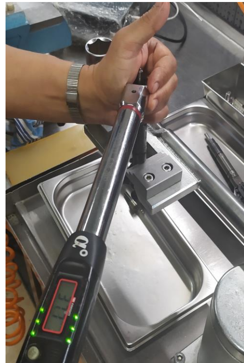
Fig. 7. Tightening the nut with a torque wrench
