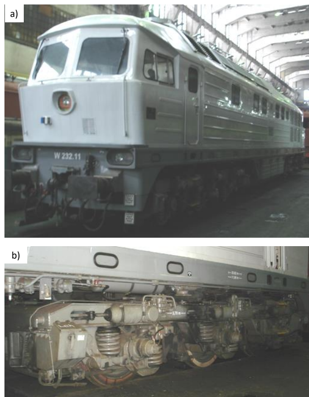
Fig. 1. View of the BR232 diesel locomotive – a), view of the bogie with the suspension system, power transmission and braking system – b)
