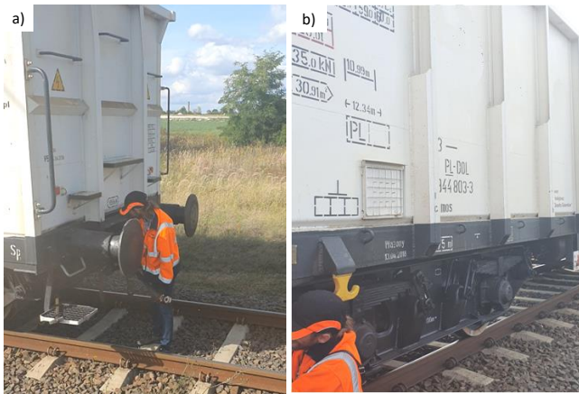
Fig. 5. View of the last wagon after the tests: a) the railway inspector conducts a simplified test of the braking system operation, b) the railway inspector evaluates the technical condition of the wagon
