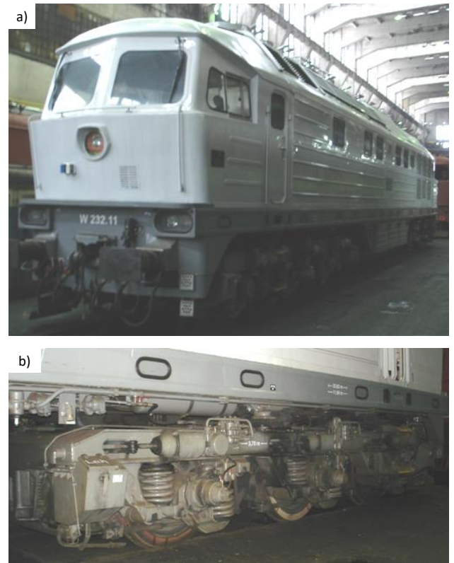
Fig. 1. View of the BR232 diesel locomotive – a), view of the bogie with the suspension system, power transmission and braking system – b)
