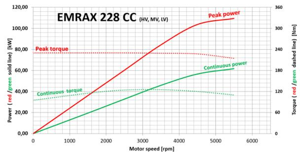
Fig. 3. External characteristics of the EMRAX 228 motor [13]
