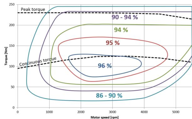
Fig. 4. Efficiency map of the EMRAX 228 motor [13]
