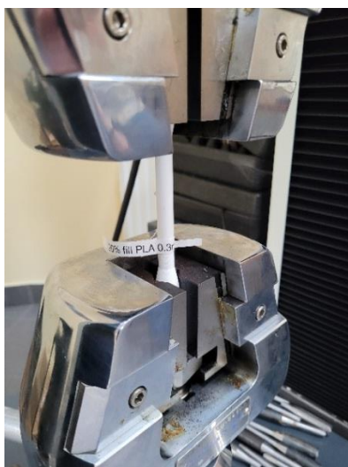
Fig. 5. Jaws of the QC-503M2F Universal Testing Machine, general view
