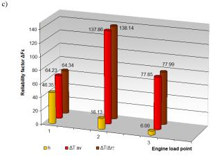
Fig. 14. Amounts of reliability factor  $\Delta F$  for univariate analysis of the impact of modifications of engine load P and structure parameters: field of the active section of intake airflow  $A_{inj}$  (a), opening pressure of fuel injector  $p_{inj}$  (b), and compression ratio  $\epsilon$  (c) on amounts of defined diagnostic tools (h,  $\Delta T_{av}$  and  $\Delta T/\Delta \tau \uparrow$ )
