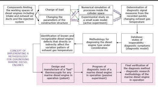
Fig. 13. Diagram of the realization of research of heat-flow processes in the exhaust gas duct for diagnostics of selected parts of systems of a ship engine
