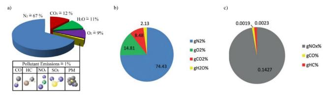
Fig. 4. Composition of exhaust gas from a diesel-powered car engine (a) [41]; gaseous chemical composition of the exhaust of the ship engine powered by RMD 80 marine fuel: mass fractions of basic (N<sub>2</sub>, O<sub>2</sub>, H<sub>2</sub>O) and harmful (CO<sub>2</sub>) chemical compounds (b); mass fractions of toxic compounds (NO<sub>x</sub>, CO, HC) (c) [25]
