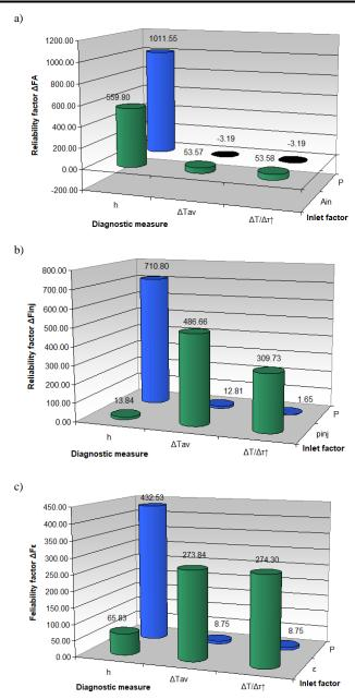
Fig. 15. Amounts of reliability factor  $\Delta F$  for bivariate analysis of the concurrent impact of engine load P and structure parameters: field of the active section of intake airflow A<sub>in</sub> (a), opening pressure of fuel injector p<sub>inj</sub> (b), and compression ratio  $\epsilon$  (c) on amounts of defined diagnostic tools (h,  $\Delta T_{av}$  and  $\Delta T/\Delta \tau \uparrow$ )
