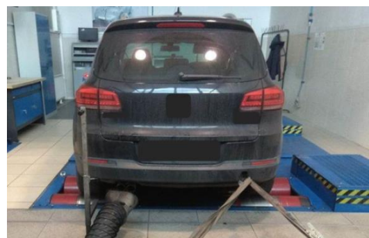
Fig. 3. Tested vehicle on the chassis dynamometer at the Department of Automotive Engineering, WUST
