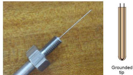
Fig. 2. Photo and cross-section of a type K thermocouple used in rapidly variable measurements
