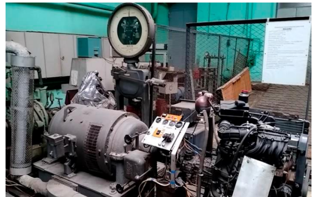
Fig. 1. Scheme of the test bench and general view: 1 – engine equipped with control and measuring devices and devices ensuring its operation; 2 – diagnostic connector; 3 – gearbox; 4 – loader/electric motor for driving the crankshaft during scrolling; 5 – pressure sensor in the engine cylinder AVL; 6 – crankshaft angle sensor; 7 – mark of the VMT; 8 – probe of the Sauermann Si-Ca 230 gas analyser; 9 – K-Line adapter; 10 – PCI L-Card 783-86 ADC board; 11 – amplifier
