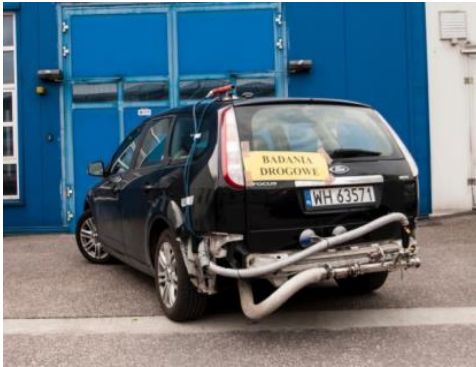
Fig. 3. Test vehicle with Semtech DS test equipment installed
