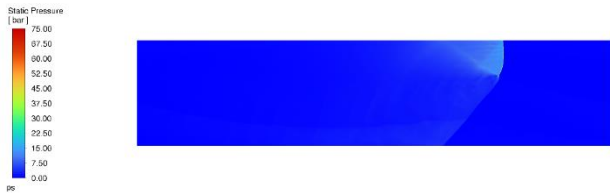
Fig. 25. Pressure distribution within the domain at t = 3 ms (AMR turned on)
