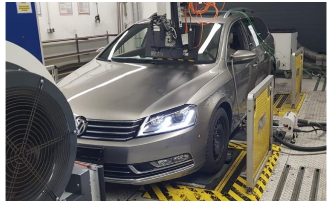
Fig. 6. Vehicle ready for the NEDC cycle
