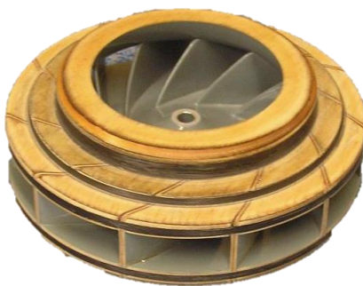
Fig. 2. Compressor rotor of the FD3-64 engine [13]
