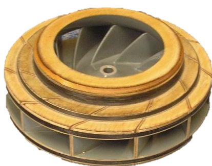
Fig. 2. Compressor rotor of the FD3-64 engine [13]
