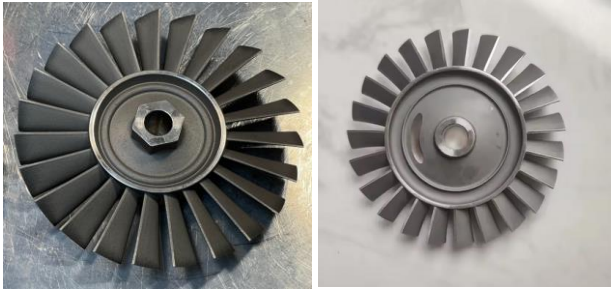
Fig. 18. Fanjet vs. conventional turbine design – 66 vs. 97 mm turbine wheel
