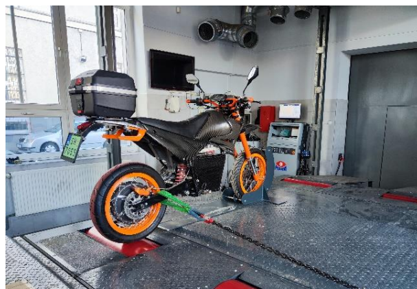
Fig. 3. View of an electric motorcycle during the dynamometer test
