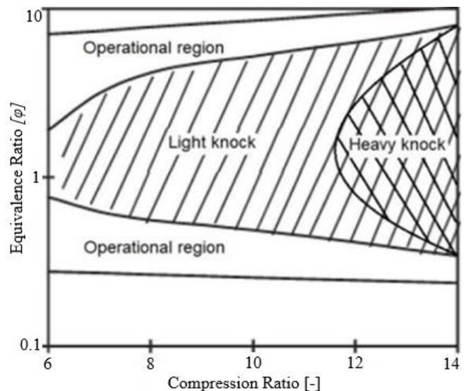
Fig. 13. Hydrogen combustion regions in SI engines [24]
