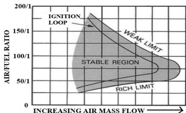
Fig. 2. Combustion stability limits [4, 7, 8]
