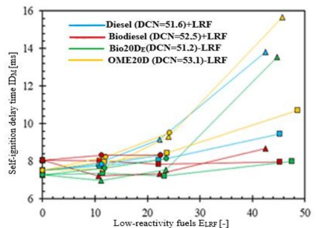
Fig. 8. Diesel and biodiesel's primary ignition delay times, BIO20D and OME20D with H<sub>2</sub>, NH<sub>3</sub> and CH<sub>4</sub> additives [17]
