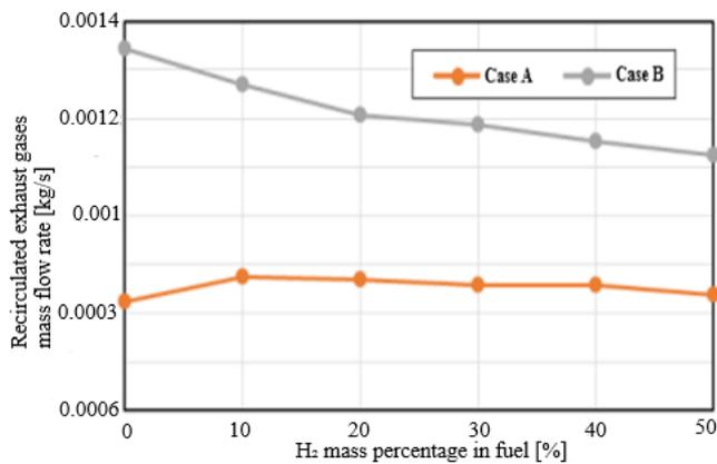
Fig. 12. Recirculated exhaust gas mass flows [12]
