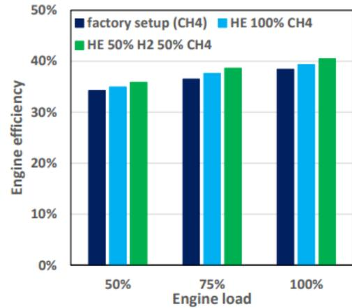
Fig. 20. Perkins engine efficiency depending on engine load [35]
