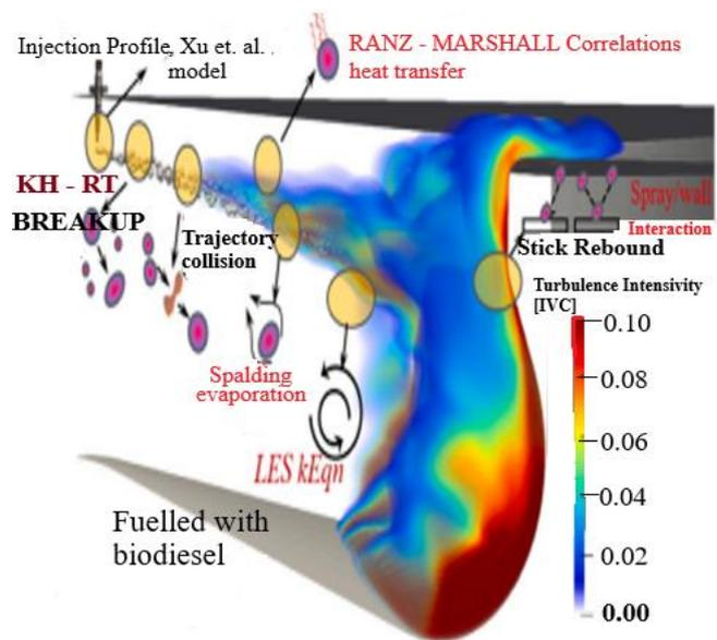
Fig. 16. Simulation models used in engine operation modelling [43]
