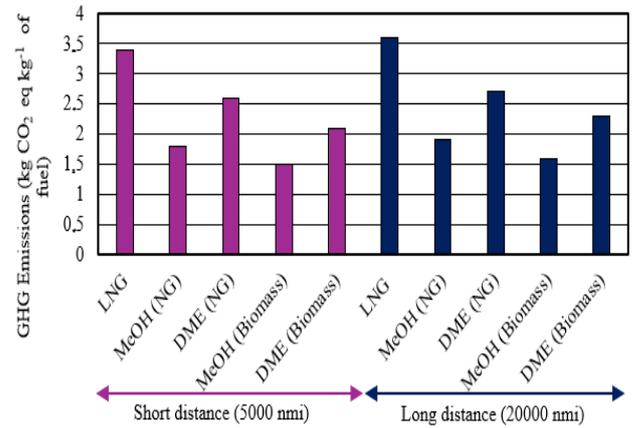
Fig. 26 Total greenhouse gas emissions per unit mass from the manufacture, usage, and transportation of methanol, DME, and LNG across short and long distances [1]
