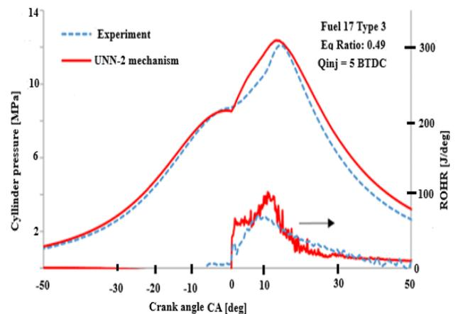
Fig. 27. calculated and experimental cylinder pressure and heat release rate curves for micro pilot initiated n-heptane syngas combustion in a dual fuel engine; air-fuel ratio – 0.31; injection timing – 13° [34]
