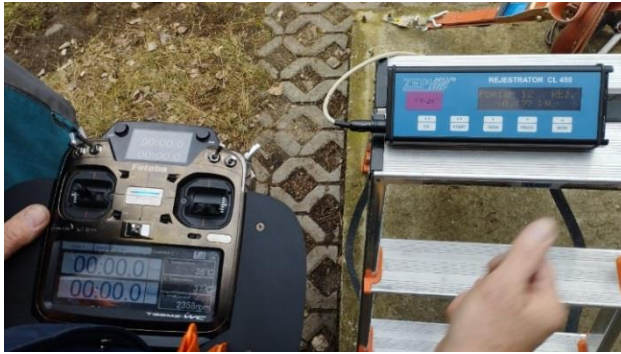
Fig. 11. Preliminary measurements on the test stand – sample measurement 1 (cylinder head 1 – 36°C, cylinder head 2 – 37°C, crankshaft speed 2358 rpm, measurement displayed on the recorder 122 N; after scaling, the thrust force value is 95.68 N)
