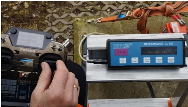
Fig. 12. Preliminary measurements on the test stand – sample measurement 2 (cylinder head 1 – 35°C, cylinder head 2 – 42°C, crankshaft speed 4952 rpm, measurement displayed on the recorder 481 N; after scaling, the thrust force value is 377.25 N)
