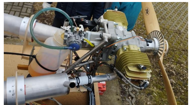
Fig. 3. Arrangement of the measurement assemblies on the test stand and integration of the exhaust system
