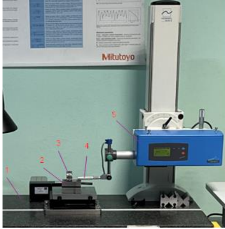
Fig. 5. The measurement of the roughness parameters for the bore surface of a toothed pulley using the measuring unit Hommel-Etamic W40. 1 – profilometer measuring table, 2 – measuring holder, 3 – tested toothed pulley, 4 – profilometer measuring needle holder, 5 – profilometer measuring head
