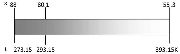
Fig. 3. The influence of water temperature on its relative electrical permittivity
