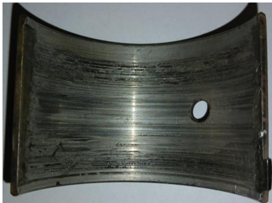
Fig. 1. Friction traces on the inner liner of the plain bearing
