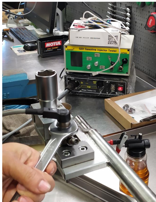
Fig. 8. GAP calibration during the tightening of the piezoelectric actuator
