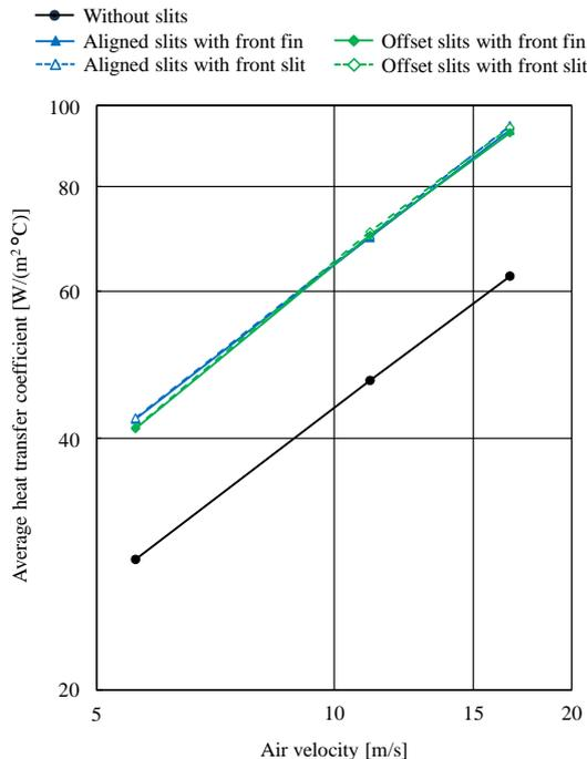
Fig. 8. Average heat transfer coefficient vs. air velocity
